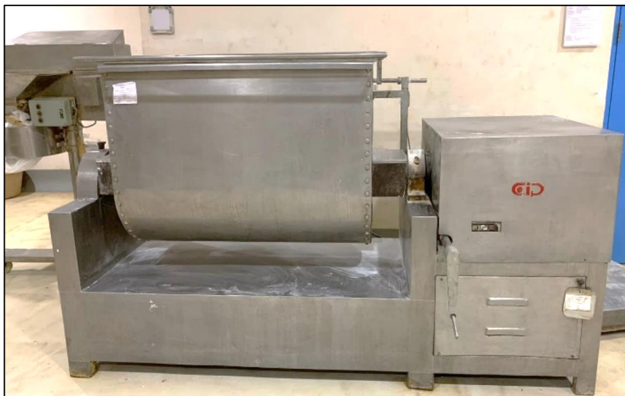
Mass Mixer Machine Use for Powder Mixer
