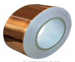
Copper Foil Tape Dxinst-0701-85-35 has a 35um smooth copper (Purity is 99.95%) foil backing with a 50um Conductive acrylic pressure-sensitive adhesive and liner. The unplated copper with conductive adhesive is a common EMI shielding tape for non- corrosive conditions.
