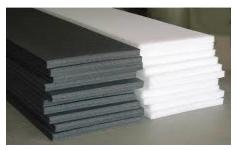
Polyurethane Foam is one of the most popular materials used in acoustic applications like DG set , Compressors, automotive industries for cushioning , anti-vibration , acoustic dash boards, refrigerators , Ac, washing machines, home furnishing such as furniture , bedding and carpet underlay, etc.
