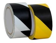
DFMT-150 is a tough plasticised PVC tape coated with an aggressive modified rubber- adhesive and reverse coated with release agent available in Yellow, Black, Green, Blue, White, Red, Black & Yellow, White & Red. Suitable for lane marking to delineate lanes and opening, hazard warning to identify potential risk area and safety zone.
