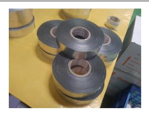
DAFT-3020 is dead-soft Aluminum Foil Tape coated with solvent based acrylic pressure sensitive adhesive with FR properties , available in with and without release liners variants. Aluminum foil tape has many uses including sealing ducts for heating, air conditioning and refrigeration, vapor barrier, sealing and masking of aircraft, masking in powder coating applications, heat reflection and dissipation applications and as an EMI/RFI shielding.
