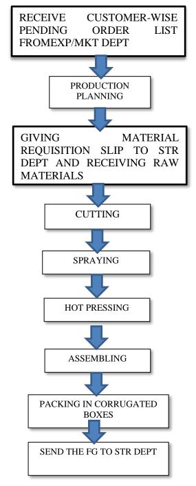
Our manufacturing process begins with procurement of raw materials such as Particle Board, Aluminium Frames,
